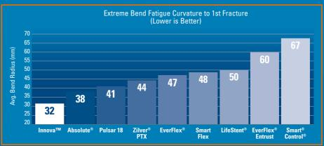
Bend fatigue curvature to first fracture measured by bend radius in 37° C (98.6° F) water bath at 5 mm diameter when average of one fracture is observed using interpolation between decreasing radius increments. Data on file. N = 3. Stents tested: 7 x 40 mm.
